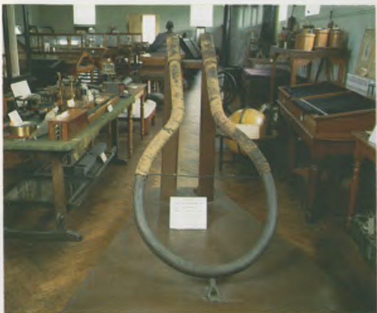
Electro-magnet invented in 1834 by Nicholas Joseph Callan (right)
